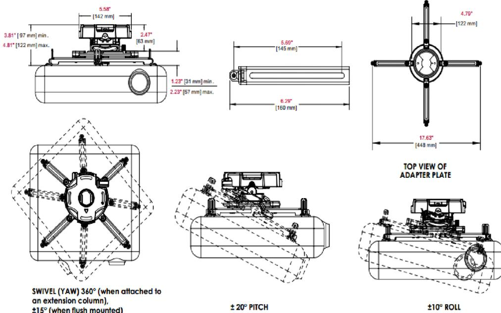
SWIVEL (YAW) 360° (when attached to an extension column), ±15° (when flush mounted)
