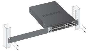
To install two half-width switches in a rack, inside and outside middle mounts and rack-mount brackets are supplied with the switches:
