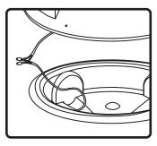
6. Attach signal wire to wire leads. Use wire nuts provided. For added water proofing, grease caps are recommended.
