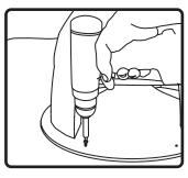
7. Set speaker enclosure on speaker base. Use tamperresistant stainless-steel screws to attach speaker to base (driver tip and screws provided).
