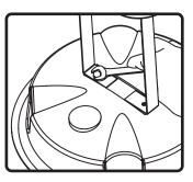
2. Attach inground/security brackets to speaker base using stainless-steel bolts.
