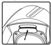
To enhance bass performance, remove port cover on the underside of speaker enclosure. Warning: Removing the cover will expose internal components to humidity and other potentially corrosive elements.
