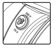
5. Select the tap position by removing the rubber plug to access rotary switch. Switch is preset to maximum tap setting in 70.7 V mode (64W XT850, 32W XT550). Select desired setting and reinsert rubber plug.
