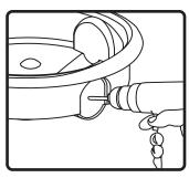
1. If needed for daisy chaining drill speaker base and install second liquid-tight strain relief (not included).
