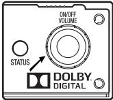
1. Turn the SB335 on by pressing the on/off button. The LED will turn white when on.
