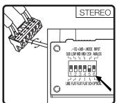
2. For 2 channels (Stereo) connect your speakers to the 2 outer sets L and R terminals. Set dip switch 5 in the up position.
