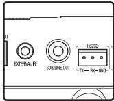
1. Connect a Subwoofer to the SB335 with an Audio RCA cable.
