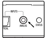
2. For analog connections connect a cable from your analog source to the analog input using a stereo 1/8"mini-jack. Set dip switch 6 in the up position.
