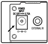
1. Connect the 32v power supply barrel connector to the power input on the SB335.
