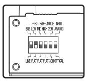
2. To boost the low frequencies set Dip switch 2 to the up position (+3dB)
