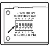
2. To use the internal SB335 crossover set to 120Hz set dip switch 1 to the up (Sub) position.
