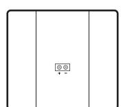
1a. Make sure the + wire is connected to the plus or red terminal on your speaker and the – to the negative or black terminal on the speaker.
