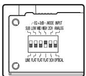
4. To boost the high frequencies set Dip switch 4 to the up position (+3dB)
