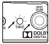
4. Press and hold the on/off button on the SB335 until it starts blinking purple (approximately 5 sec).
