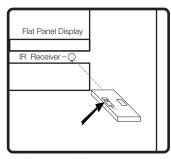
5. Point the TV remote at the IR receiver and press the volume up button 3 times. The purple LED will blink 3 times rapidly.
