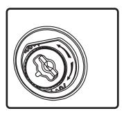
1. Select the tap position by removing the rubber plug on grille to access rotary switch. Switch is preset to maximum tap setting in 70.7 V mode. Select desired setting and reinsert rubber plug. Note: The grille-mounted tap switch cover is keyed; be sure flat edge of plug lines up with flat edge of hole in grille.
