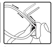
8. Adjust speaker hanging height with SpeedClamp™ mechanism. Pull to tighten & insert release key (small hex wrench) into SpeedClamp ™ as shown to loosen or adjust.
