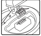
**11.** Insert 4-pin Euroblock plug into Euroblock jack on rear of speaker. Connectors are keyed for polarity.
