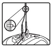
12. Use zip or twist-lock ties to secure safety cable & signal wire to main hanging cables. Cable cover available for asthetic applications (SLT-10).
