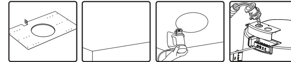
1. Nail or screw bracket to joists. Secure conduit/signal wire away from hole in bracket.
