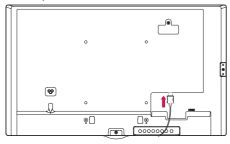
2 Mount the speakers by using screws as shown below. Make sure the power cable is disconnected before making a connection.
