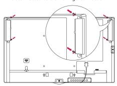
3 Then connect the speaker cable. After installing your speakers, use holders and cable ties to organize the speaker cables.
