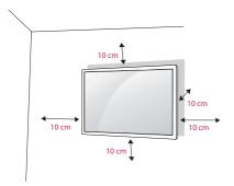
To install your monitor on a wall, attach a wall mounting bracket (optional part) to the back of the monitor.
