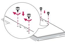
Ose the screws to secure the stand to the back of the product as shown below.
