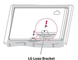
2 After removing the screw, remove the LG Logo. When re-attaching the LG Logo, repeat the process in reverse order.
