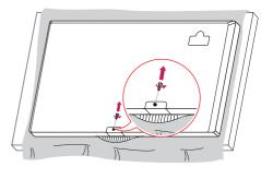
2 After removing the screw, remove the LG Logo. Attach the LG Logo Bracket with a screw, aligning it with the hole on the right side.
