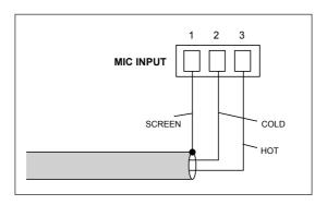
The MA80's microphone pre-amplifier is an electronically balanced, transformerless design configured for optimum low noise performance. The input impedance is greater than 2 kohms and is suitable for microphones in the 200 ohm to 600 ohm range. The microphone signal path includes a fixed high-pass filter. This attenuates the response below 100 Hz, which helps to reduce the effects of microphone handling noise.
