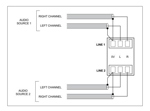
The two line inputs are summed together internally: however, note that Line input 1 can be configured to have priority over Line input 2, see "Line 1 Priority" on page 21.
