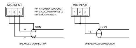
$15\,V$  phantom power is available at the mic input, and is activated by setting internal jumper JI to the ON position. See "PCB layout diagrams" on page 30 for further
