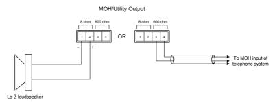
Before using the MOH/Utility output with a telephone system, it is recommended that the system manual is consulted to check suitable audio levels and any other compatibility issues.
