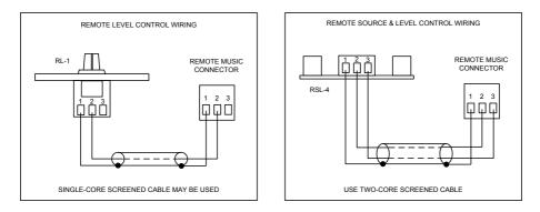
Use two-core (RSL-4/RSL-4A or RL-1/RL-1A) or single-core (RL-1/RL-1A only) screened cable to connect the remote level plate. The maximum recommended cable length is 100 m.
