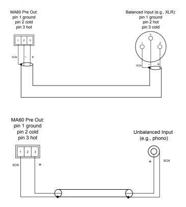
All the unit's controls and settings on the front and rear panels (levels, source selection, priority settings, etc.) are effective at the Pre Out. However, note that neither the switchable 65 Hz high pass filter nor the fitting of an optional loudspeaker EQ card have any effect on this output.
