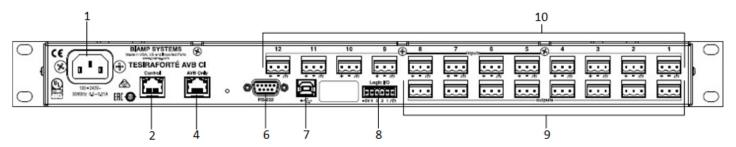
Figure 8 TesiraFORTÉ CI AVB model (Rear Panel View)
