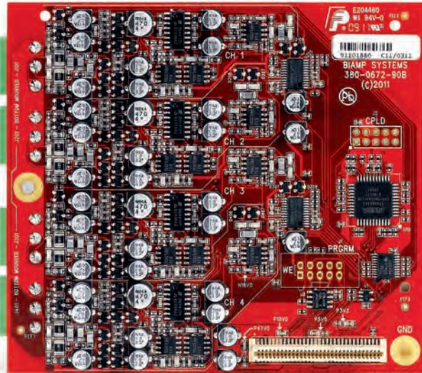
The Tesira® EIC-4 is an expander card with 4 analog input channels for use with Tesira EX-MOD device. The EIC-4 is one of three optional cards that can be mounted in Tesira EX-MOD. Each EIC-4 provides 4 channels of mic/line level audio input. The inputs are electrically balanced and provided on plug-in barrier strip connectors. Software control of each input includes gain with clip indicator, +48V phantom power, mute, level, and signal invert.
