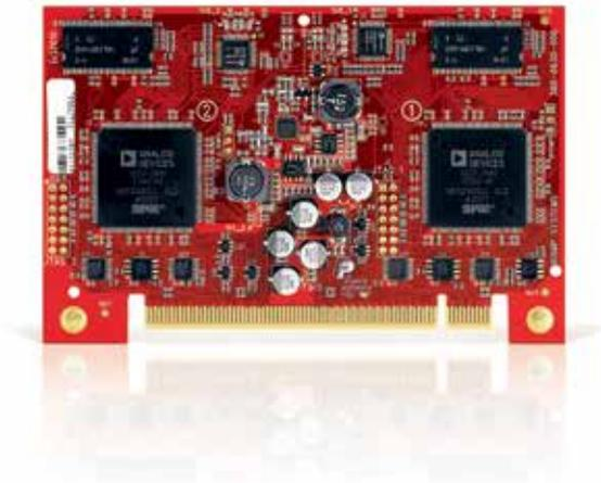
The Tesira DSP-2 card is a modular digital signal processing card for use with Tesira SERVER and SERVER-IO devices. DSP-2 cards provide signal processing power to a Tesira system. As the necessary processing increases for larger systems, DSP-2 cards can be added in the field or at the Biamp factory. The Tesira SERVER can accommodate up to eight DSP-2 cards while SERVER-IO can support up to three.
