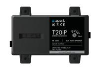
The T20IP is a small built-in 100 volt line transformer, designed to make it possible to convert a standard 8 ohms loudspeaker into a 100 volt line speaker with selectable power taps (2.5 - 5 - 10 and 20 watts in 100 volt).
