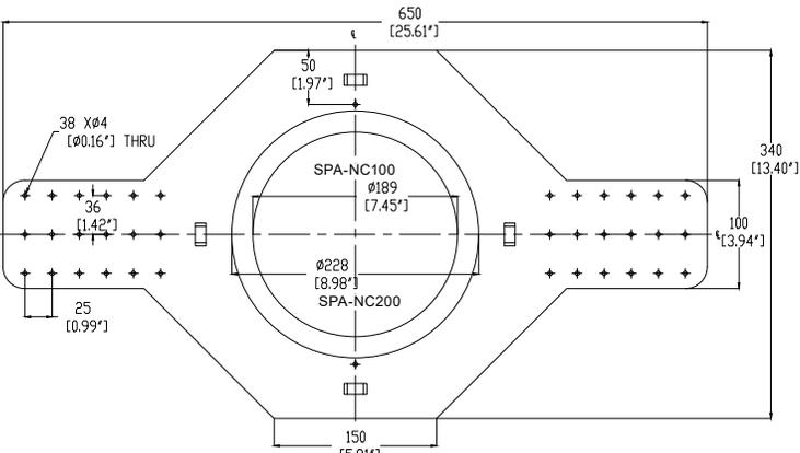
Exterior dimensions and hole placement are shared on the 3 drawings at left. The ID of the hole cutout is noted for each model.
