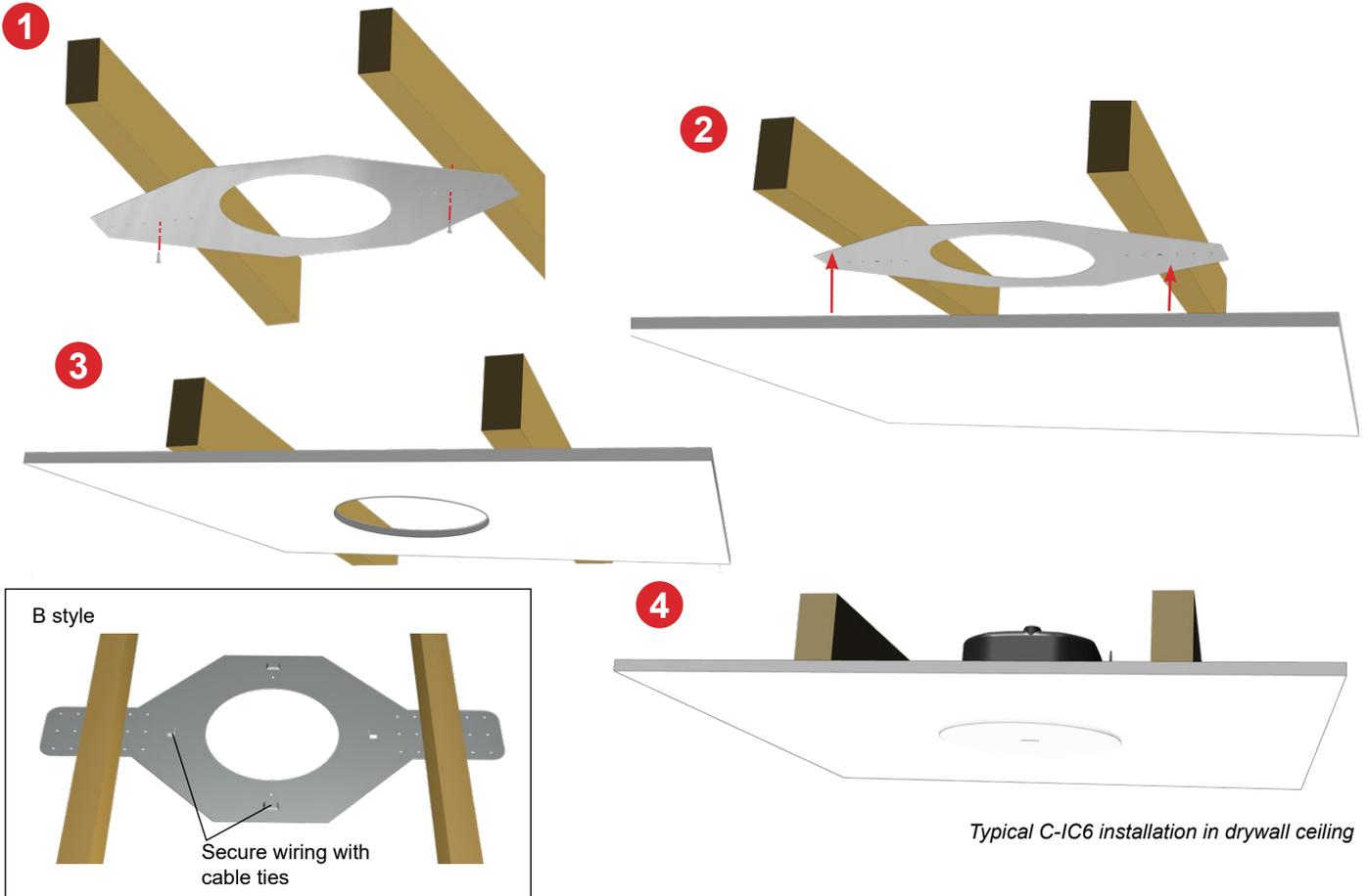
*Typical C-IC6 installation in drywall ceiling*
