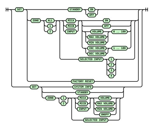
Figure 16. RS232 Text Command Diagram
