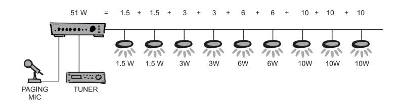
In fact working with 100V loudspeakers is rather simple, when done in the right way. Each 100V loudspeaker has a 100V transformer which can be set to a certain power, for example: 1,5 3,6 or 10W. As the example shows, the sum of all loudspeaker settings should never exceed the amplifier's power specifications.
