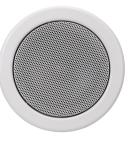
The Apart EN-CM5T6 is a 5.25" built-in ceiling speaker made of powder coated steel (RAL 9010 equivalent), equipped with a high efficiency full range speaker and a multi tap 100 volt transformer, all certified according EN 54-24.
